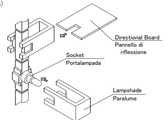
※The illustration shows the fixture, omitting partial detail.
